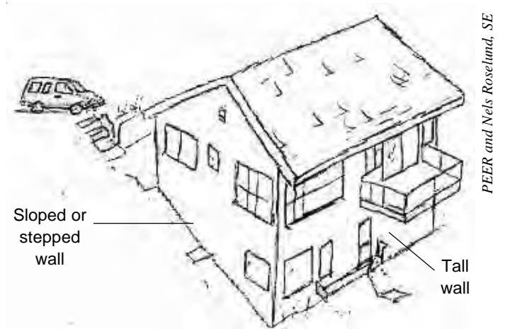
Figure 24 - Hillside homes with sloped and tall walls or posts require special engineering.
